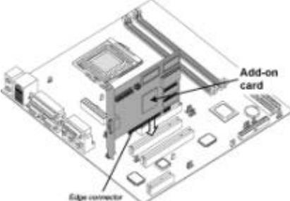
An isometric diagram of a computer motherboard. A grey add-on card is shown being inserted into a slot. A label 'Add-on card' points to the card, and a label 'Edge connector' points to the bottom edge of the card. The card is shown partially inserted into the slot, with a metal bracket on its side. |
