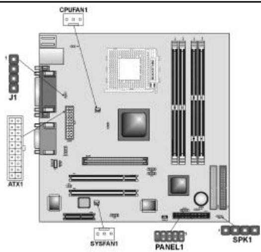
4. Connect the case switches and indicator LEDs to the **PANEL1** header.
