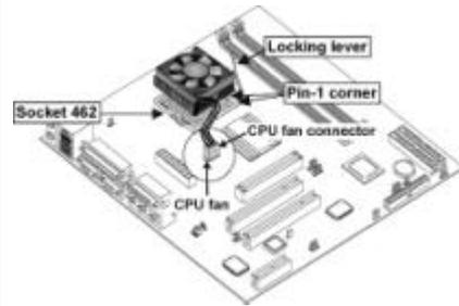
**Note:** CPU fan and heatsink installation procedures may vary with the type of CPU fan/heatsink supplied. The form and size of fan/heatsink may also vary.
